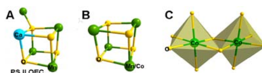
Figure 1. (A) OEC active site of PS II (PS II-OEC site). (B,C) Structural models for synthetic WOCs possessing a M 4 O 4 cubane-type topology (B) and an edge-shared octahedral topology (C).
